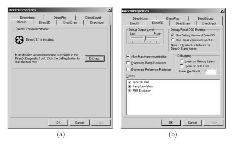
Figure 22.2: DirectX Control Panel Applet. (a) The DirectX page. (b) The Direct3D page.
