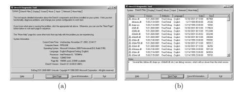
Figure 22.1: DirectX Diagnostic Tool. (a) The System page. (b) The DirectX Files page.
