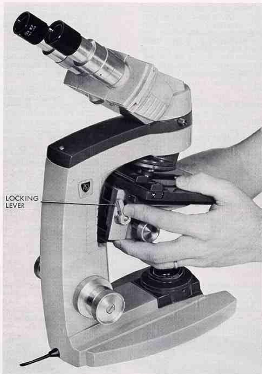
Figure 12. Removal of Stage Assembly
