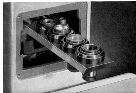
Photographic eyepieces are mounted on dovetail slide within the instrument. Operated by external control, they are easily accessible through camera aperture. (Normally, it is not necessary to remove side plate of the instrument.)
