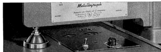
Rubber shock absorbers, located between the instrument assembly and the desk unit, effectively deaden high-frequency vibrations. These are supplied as standard.
