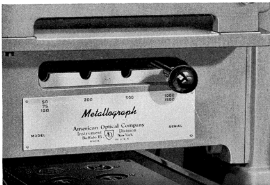
Control lever above A.S.T.M. magnification scale permits instant selection of desired photographic eyepieces.
