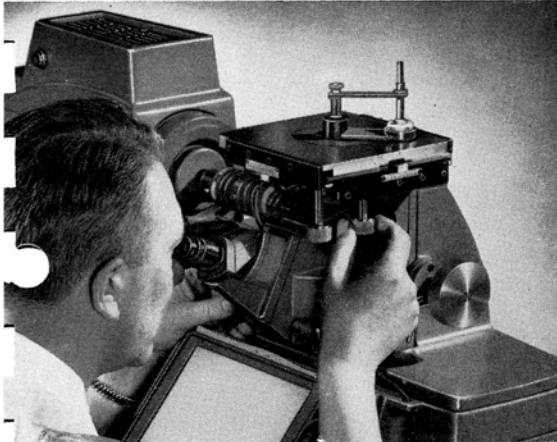
Close-up shows large square graduated ball-bearing mechanical stage.
