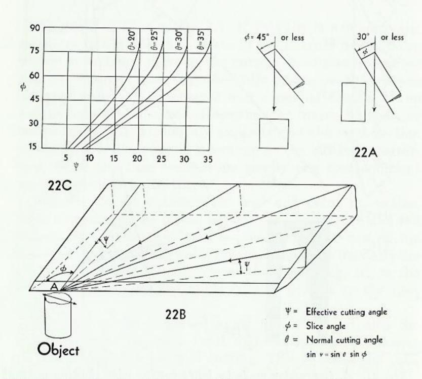
Fig. 22. A. Showing slice angle  $(\emptyset)$  for square and rectangular blocks. B. Decreased wedging with small slice angles. C. The relations between them plotted with permission from data of Preston (1933).
