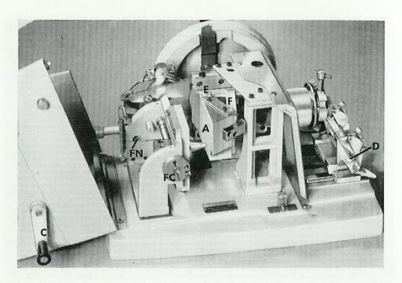
Fig. 6. AO Spencer Microtome with thin cutting attachment (A).
