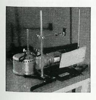
Fig. 34. Interferometer for measuring the thick-ness of sections.
