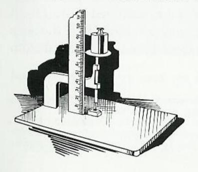
Fig. 27. Penetrometer for measuring hardness of specimens.
