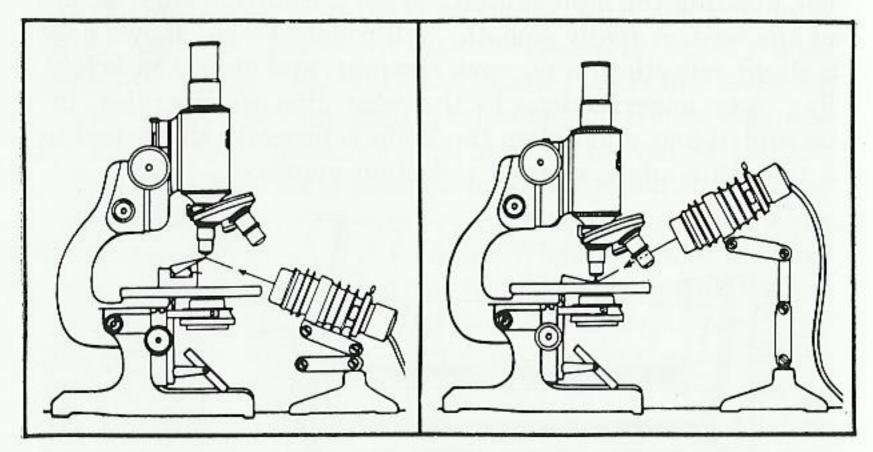
Fig. 14. A. Method for examining sharpness. B. Method for examining facet polish. (From Richards, 1950.)
