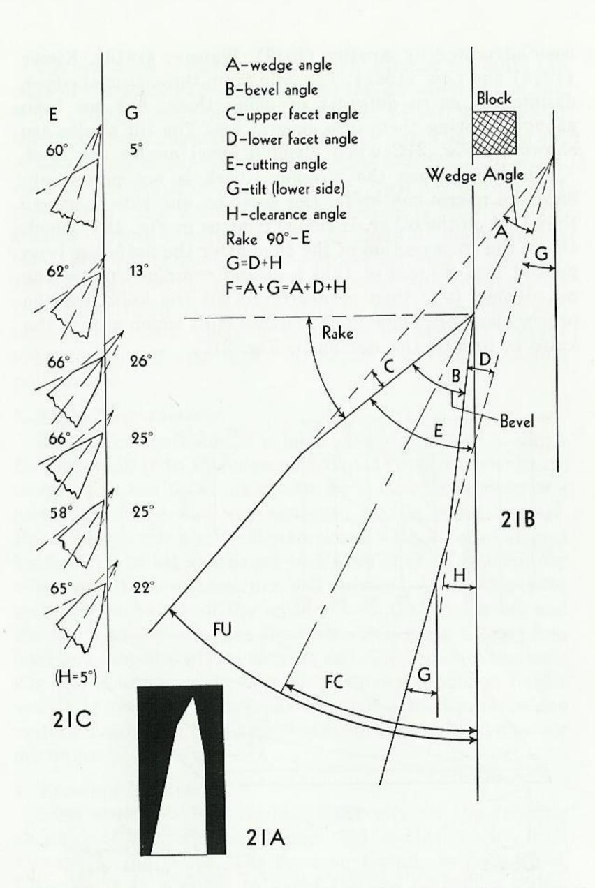
Fig. 21. A. Impression made by knife cutting edge showing unequal sharpening. B. Geometry of knife edge angles. C. Rake and tilt angles for a clearance angle of 5° for proper placing of knives with unequal facets.
