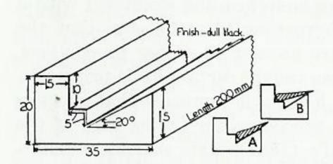
Fig. 13. Block for supporting microtome knife (dimensions in mm). A. Position for examining sharpness. B. Position for observation of polish.
