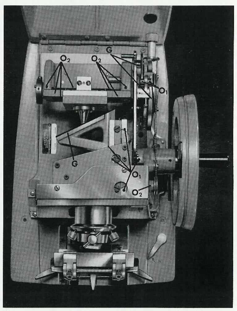
Fig. 7. Lubrication diagram for 820 Microtome.
