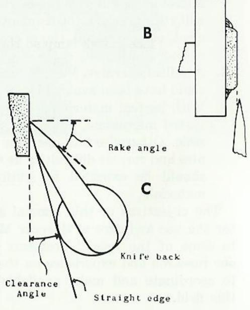
Scored, grooved, smeared and deformed sections are often caused by a dull knife. Regular, lengthwise scratches, and splits in sections are usually caused by a defect in the knife edge, although they may result from dirt or hard material in the specimen. Moving the knife to an unused region, or replacing with a sharper knife may restore good sectioning.
