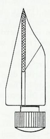
Fig. 33B. Proper position of blade in holder.
