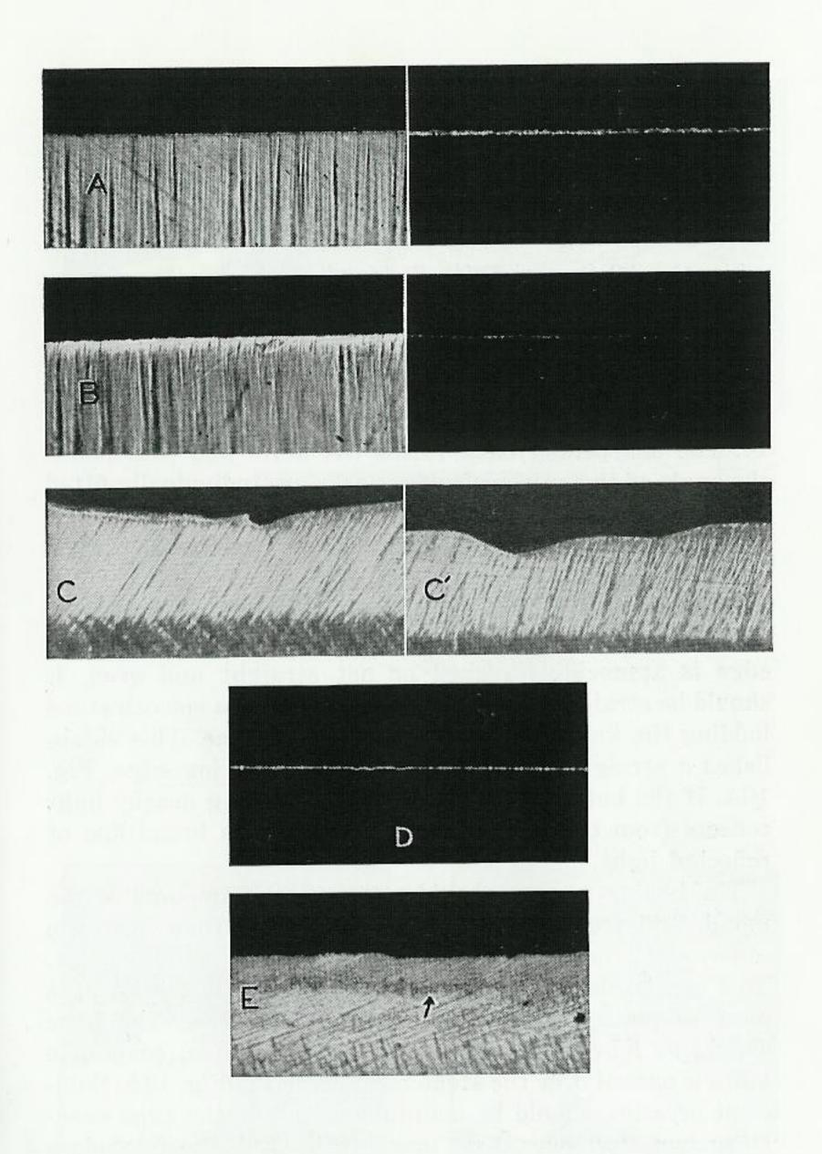
Fig. 17. Photomicrographs of edges which will not cut satisfactorily to show what to avoid. Poor edge (A) rounded by stropping (B) into line. C. Old nicks rounded by stropping. D. Wavy edge. E. Edge burned at arrow from excessive stropping.
