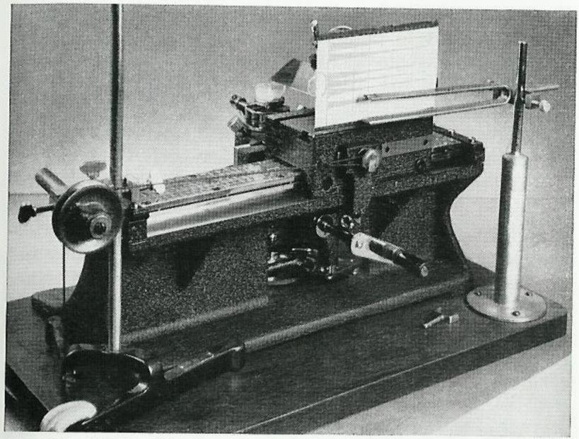
Fig. 36. Sliding Microtome arranged for measuring the resistance to cutting.
