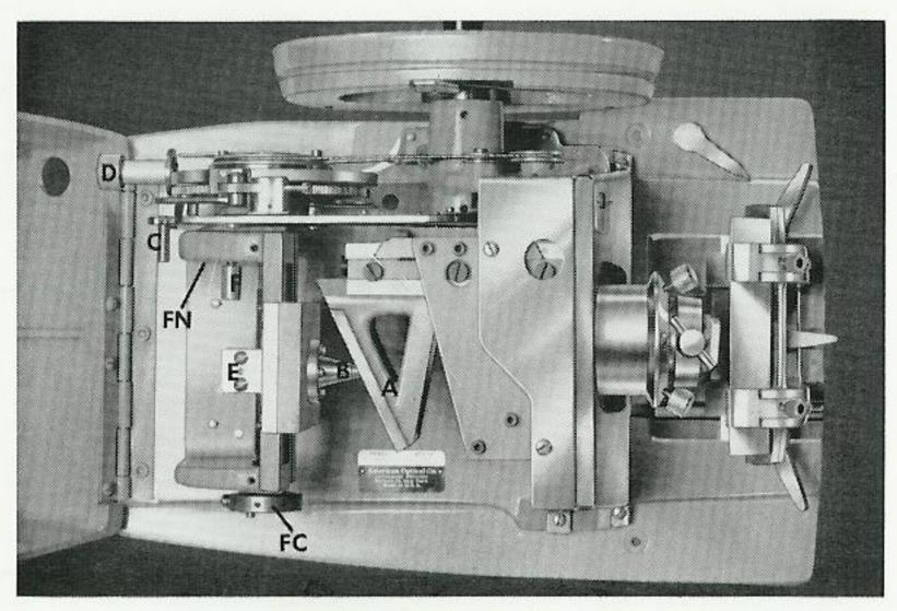
Fig. 5. Top view of uncovered 820 Microtome.
