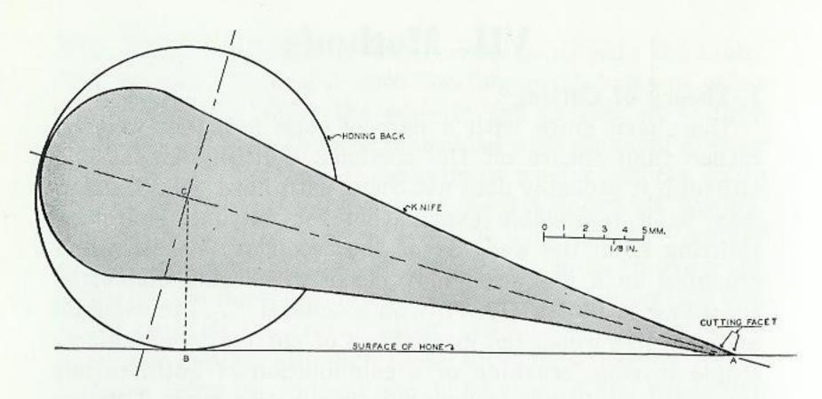
Fig. 20. Knife and honing back drawn to scale to show extent and formation of the cutting bevel and facets.
