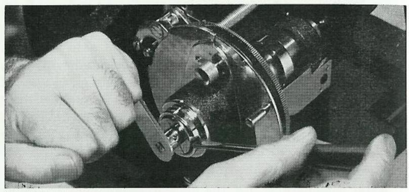
Fig. 10. Tightening the thrust nut on the feeding mechanism of figure 9.
