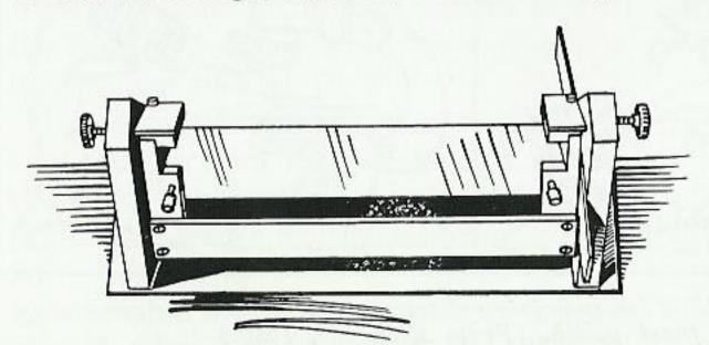
Fig. 12. Cradle for rotating microtome knife in the axis of the cutting edge.
