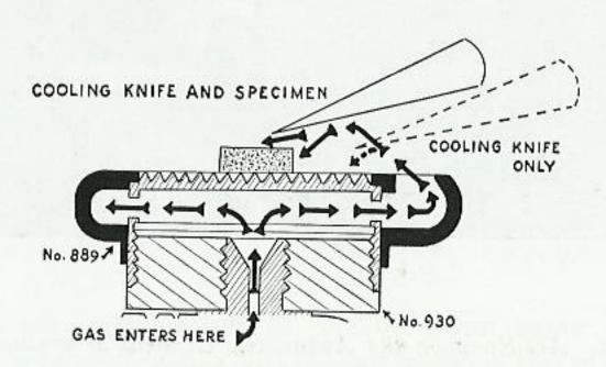
Fig. 25. Carbon Dioxide Deflector for cooling the knife and the block.
