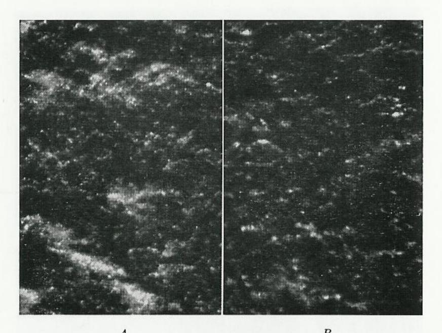
Fig. 15. Protomicrograph of (a) Yellow Belgian and (b) Blue Green hone surfaces. 100X
