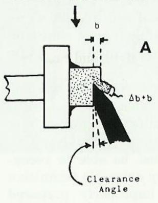
Fig. 1. A. Diagram showing clearance angle and increase in section thickness from compression. B. Wedging effect when there is no clearance angle. C. How to set the clearance angle.
