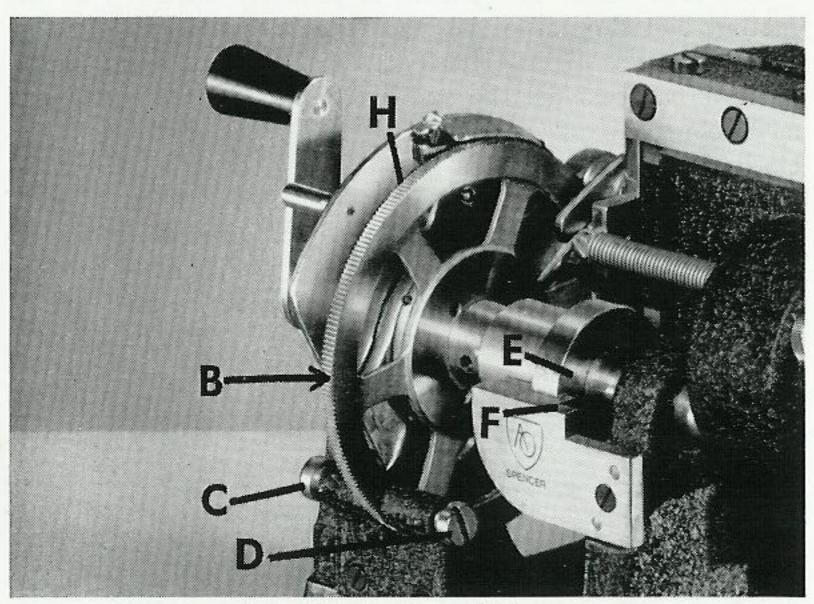
Fig. 9. Feed Mechanism of Microtome 815.
