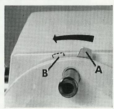
If this is a new instrument raise the cover A, Fig. 4 after pulling release knob B out, and note the slanting surface of the feed, Fig. 5A and the feed screw tip B. Remove the piece of cardboard placed between them to prevent damage during shipment. Lubricate the surface with a light neutral grease (Section D).
