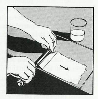
Fig.~19CFig. 19. A. Honing stroke. B. Stropping stroke. C. Glass plate method.
