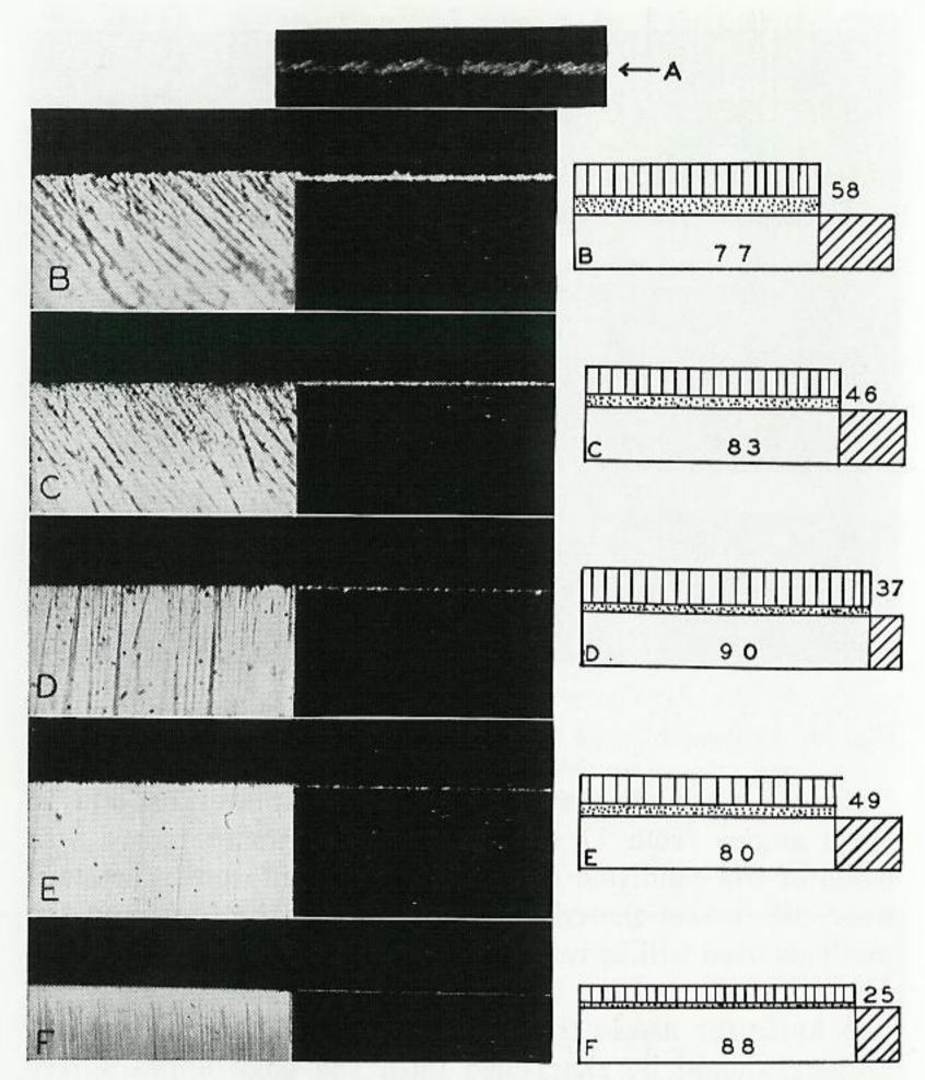
Fig. 16. Photomicrographs of microtome knife edges, light reflected from the edge and compression diagrams. (Cf. text). A. Edge flattened and straightened. B. After sharpening on Yellow Belgian Hone. C. On Blue-Green hone. D. Glass plate. E. Stropped lightly. A to E are same knife with successive treatments indicated. F. Typical factory sharpened edge.
