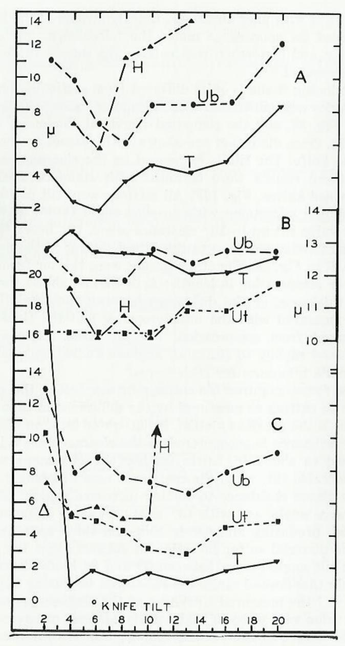
Fig. 38. Cutting resistance and compression with respect to knife tilt.
