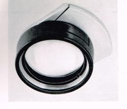
No. 323 AUXILIARY CONDENSER AND MEANS FOR ATTACHMENT. This is an extra condensing lens which, placed below the regular condenser on either substage, raises the focal point of the condenser so that the apex of the cone of light is raised about 10mm. above the surface of the stage. This makes an intense illumination at this height for drop culture work and a larger area at the plane of the
