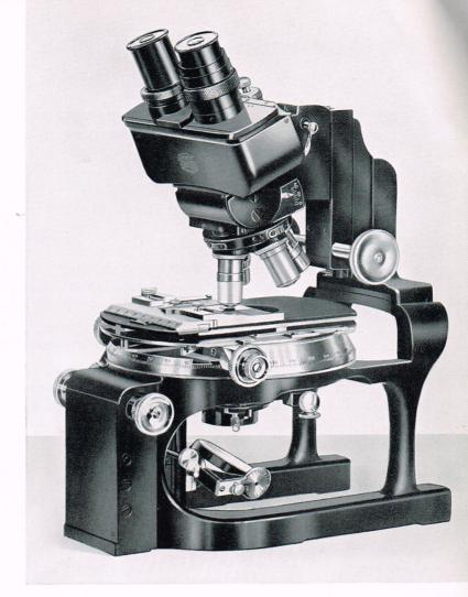
been successfully solved, using the same micrometer, bearings, etc., common to all Spencer microscopes. It affects a movement of the substage parts, together with a plate in the stage on which the slide is placed, to move it to and from the objective. The stage itself is not affected. It is sensitive, responsive and definite. Each division on the graduated fine adjustment button represents a movement of one micron. The coarse adjustment buttons are located low on the supporting arm.
