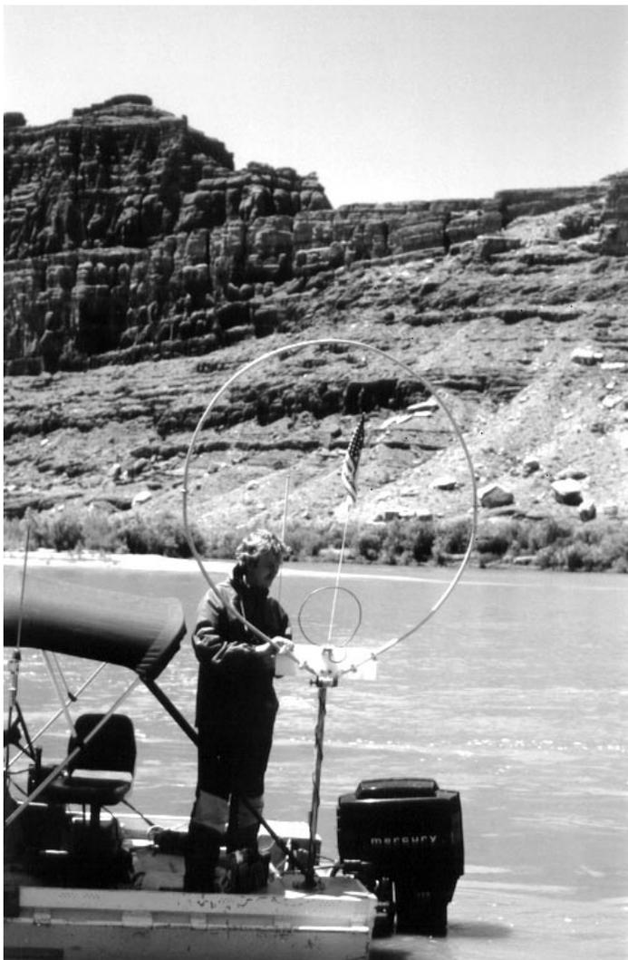
Clint, KA7OEI, makes some adjustments to the 80 Meter loop used on the Sheriff's boat
