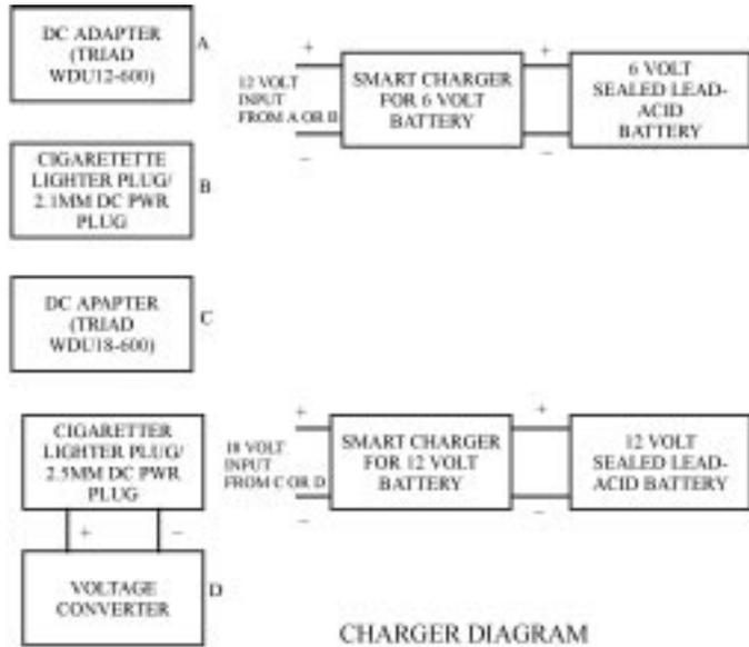
In the charger diagram, the 6 volt battery charger can be supplied with power either from the DC adapter or a power cord plugged into the 12 volt cigarette lighter jack of the vehicle.
