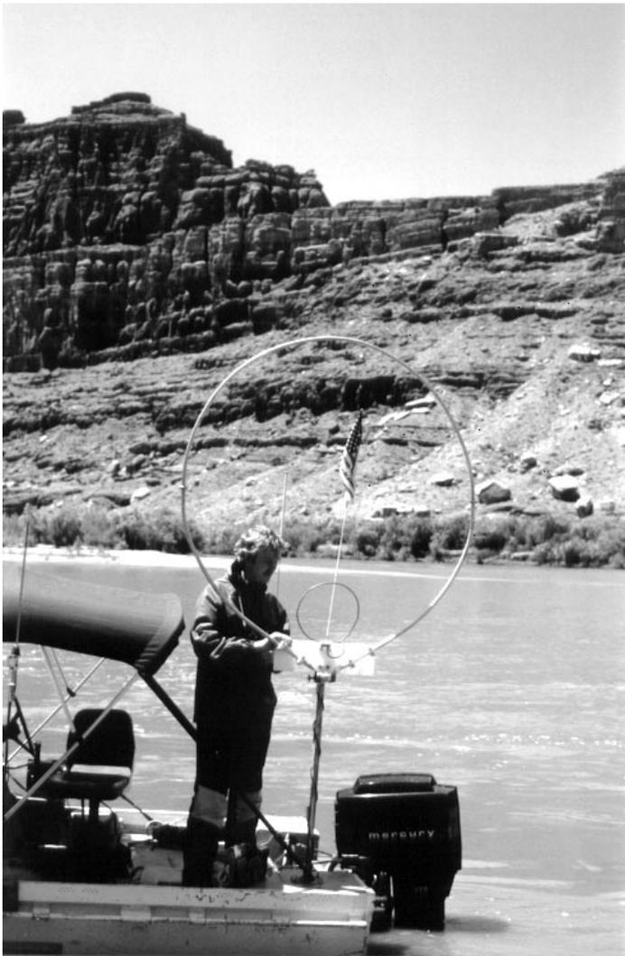
Clint, KA7OEI, makes some adjustments to the 80 Meter loop used on the Sheriff's boat
