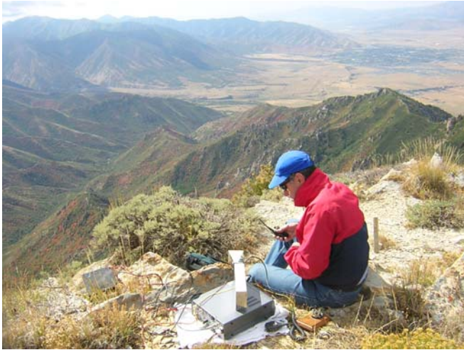
Dale, WJ7L, working Robin, WA6CDR, on Brian Head Peak, over 200 miles away. Dale's antenna is the small horn on the end of the transverter which is sitting atop his TS-2000 IF rig. See the telegraph key to the left of Dale. That is what he used to work Robin.
