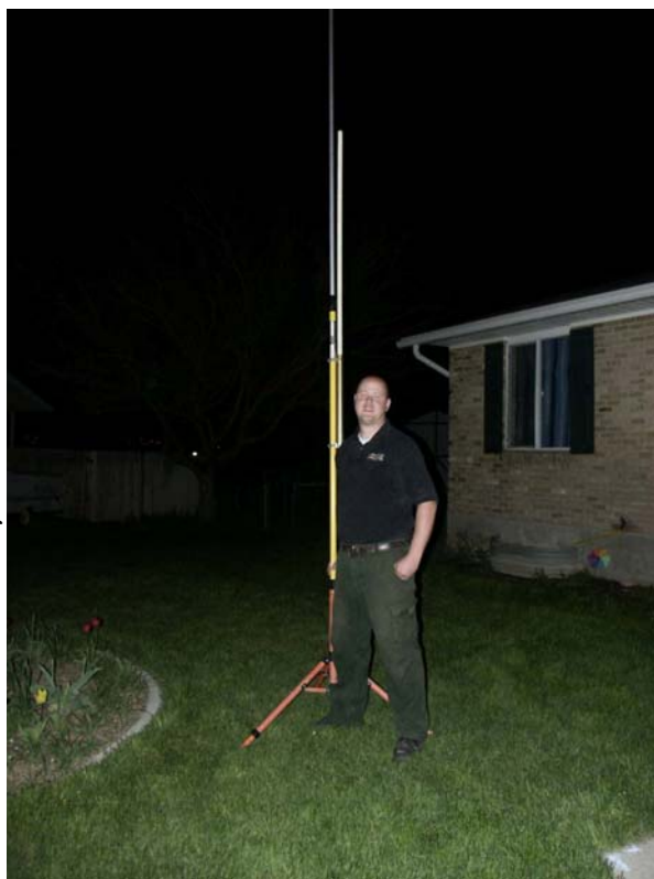
Portable dual 2-m antenna for field work (this can be deployed in about 2 minutes!)
