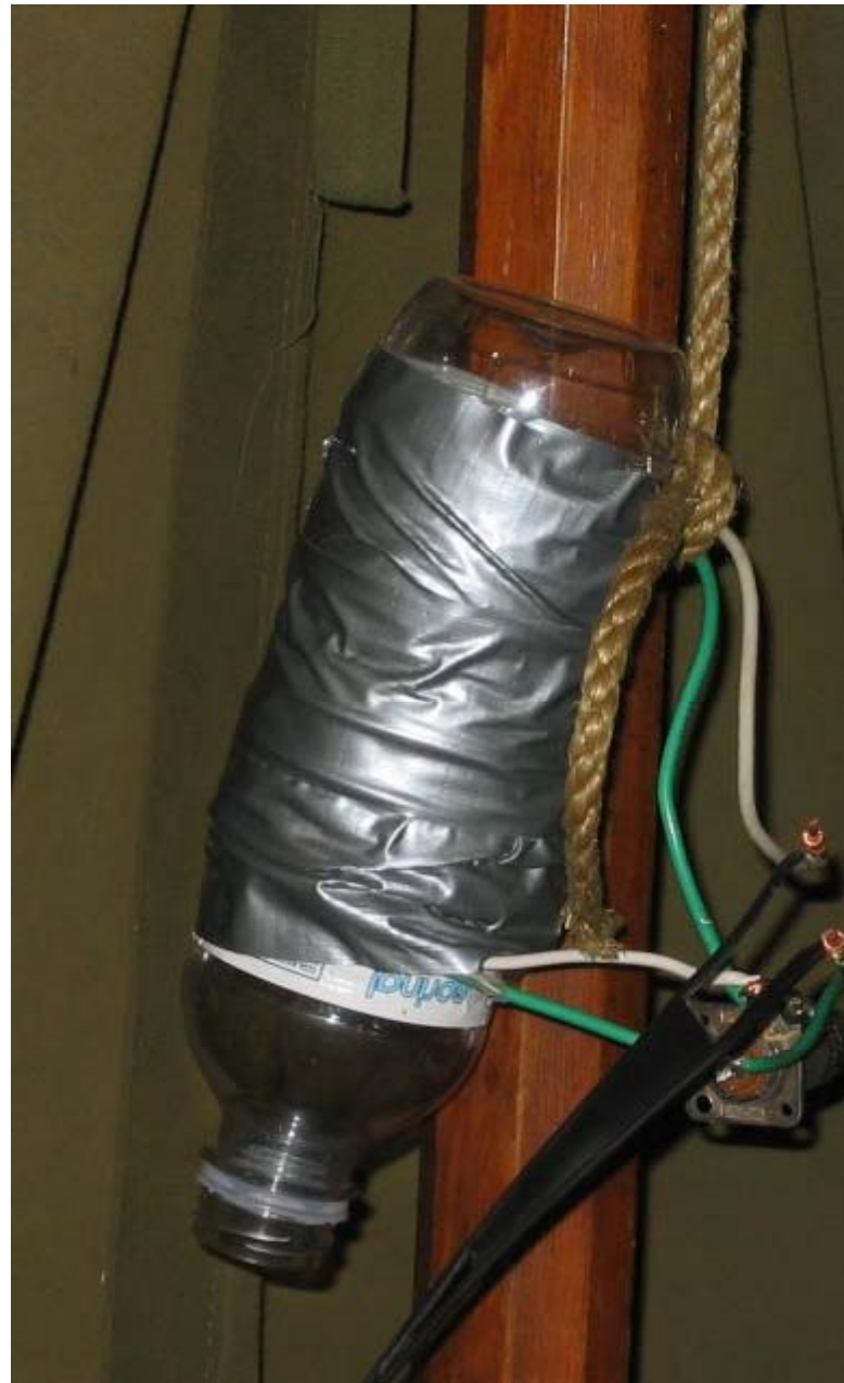
WA7X's "Bottle Balun" for balanced lines
