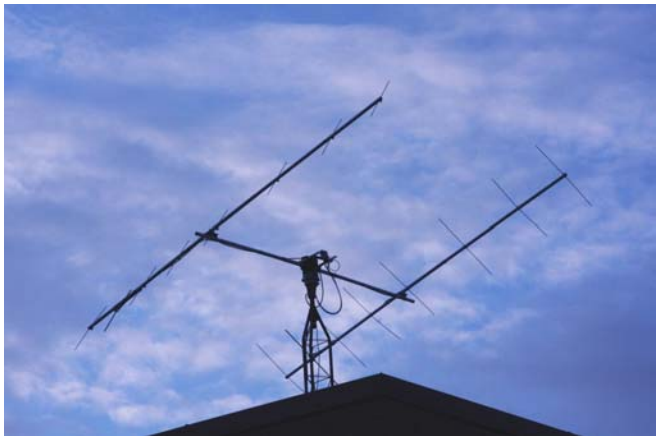
The antenna: 8 elements horizontal and vertical (Photo by Rex Estes, K7XTC)
