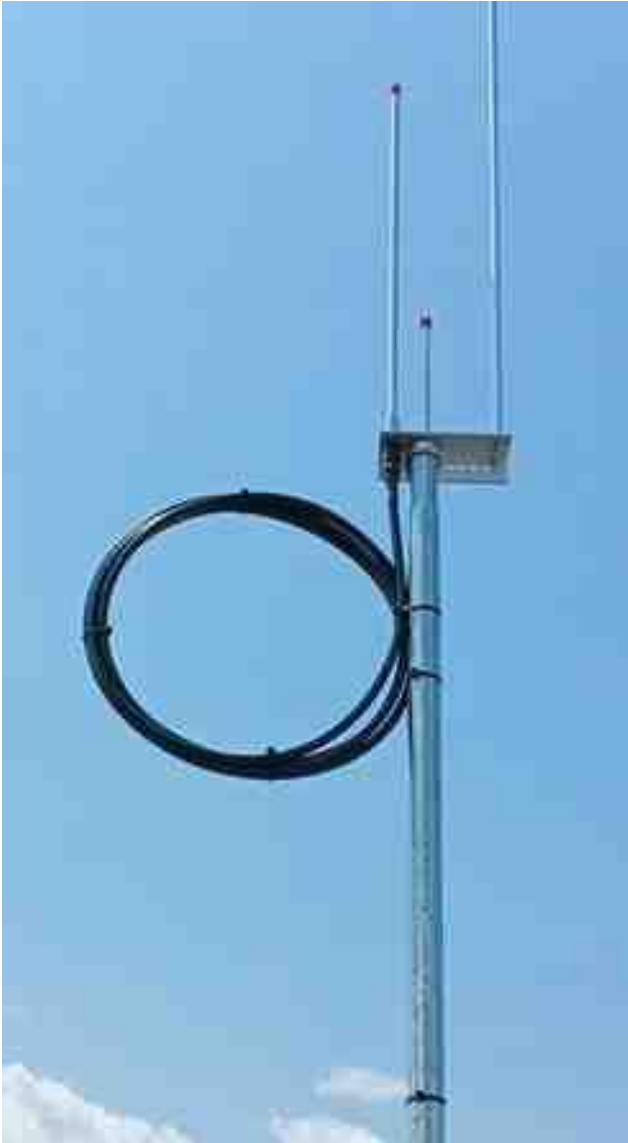
Figure 1: J-pole with RF choke made from Coax
