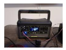
I use this to power my Kenwood TM-V71 2 meter, 70 cm rig. A two hour UARC roundtable with lots of 5 watt FM transmitting, I used less than 10% of available battery life.
