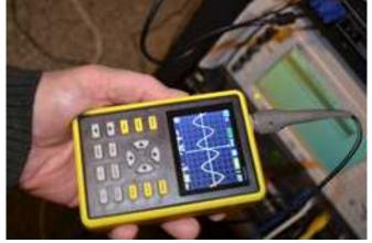
It works, a bit clumsy until you get used to its foibles. What's it good for in the shack? Audio monitoring, debugging home brew projects, HF signal monitoring, and power supply issues come to mind.
