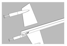
□ 20. Apply glue to the root edge of one of the triangular fins and position it along one of the lines drawn for the fins on the side of the body tube and even with the bottom of the main tube. Glue it using the same technique used on the main fins. Repeat for the other triangular fins. Allow the fins to completely dry, checking carefully to make sure they are parallel with the main body tube.
