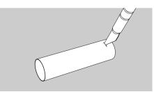
□ 7. Tie a loop in one end of the yellow Kevlar® cord (SCK-12). Insert one end of the engine hook through the loop and into the punched slit.
