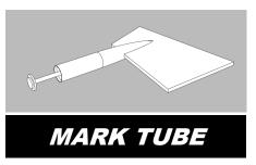
□ 18. Stand the large body tube (BT-50L) on the fin guide below and make the fin position marks on the sides of the tube. Find a convenient channel or groove such as a partially open drawer, a door jamb (as shown,) or a piece of molding. Using the channel, extend the marks the length of the tube to provide lines for aligning the fins.
