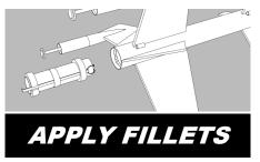
□ 25. After the fin assembly is completely dry, run a small bead of glue along both sides of each of the fin-body tube joints. Using your forefinger, smooth the glue into fillets. Allow this assembly to dry in a vertical position.
