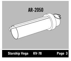
□ 9. Slide the Mylar retaining ring (HR-20) over the end of the engine tube until it is centered on the tube. Apply a bead of glue around both sides of the joint formed by the ring and tube, keeping glue off the engine hook end closest to the bottom of the engine tube.
