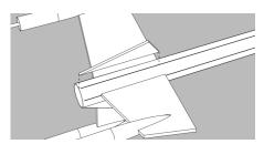
□ 21. Apply glue to the root edge of one of the small fins and position it along one of the lines drawn for the main fins on the side of the body tube and 4-5/8" from the top of the main tube. Glue it using the same technique used on the main fins. Repeat for the other small fins. Allow the fins to completely dry, checking carefully to make sure they are parallel with the main body tube.
