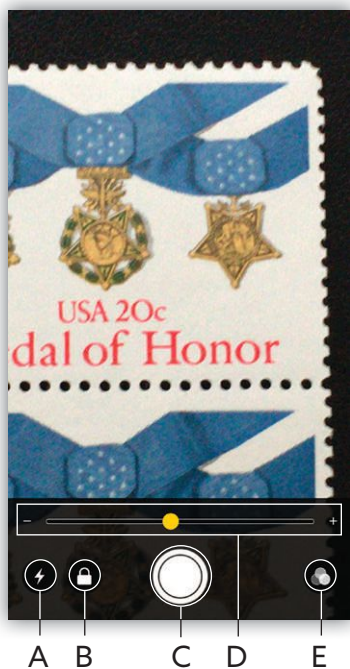
Figure 1. The Magnifier App offers the ability to use the flash for steady illumination (A), a focus lock (B), a snapshot view (C), magnification slider (D) and adjustments for contrast, brightness and color (E).
