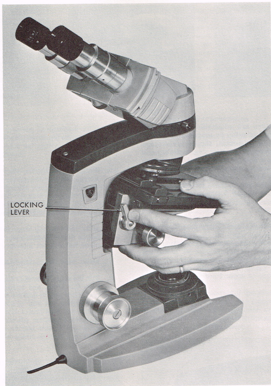
Figure 12. Removal of Stage Assembly
