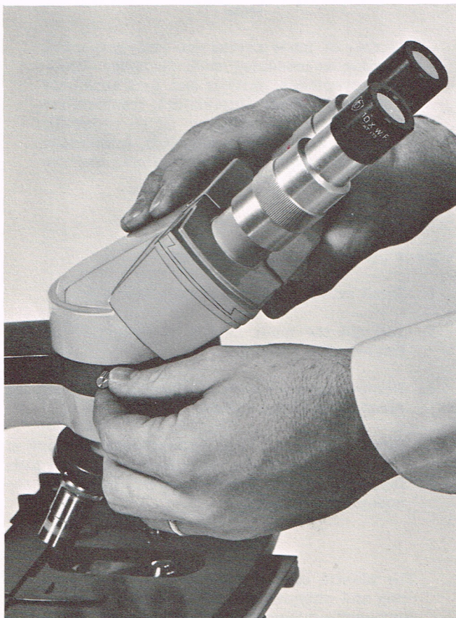
Figure 1. Attaching Binocular Body to Stand
