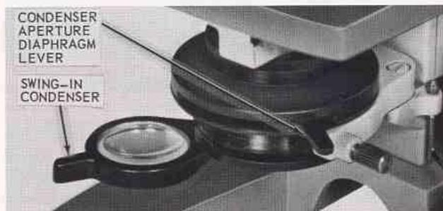
Figure 29. Substage Condenser and Aperture Diaphragm
