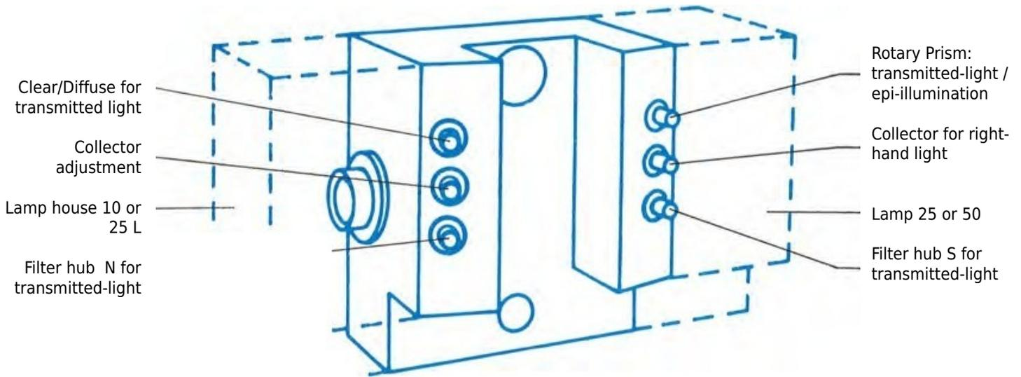
On the mirror house 2, two bulbs of your choice can be attached, e.g., the halogen lamp on the left, and the lamp house 25 or 50 on the right. This allows:
