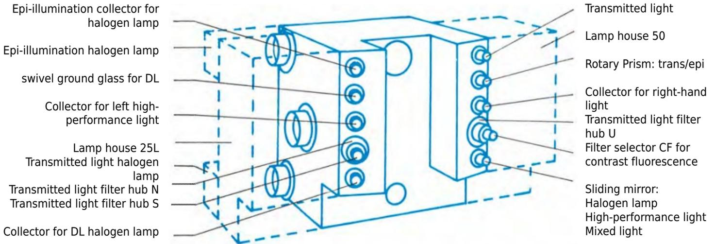
On the mirror-house 4, a halogen lamp can be used for both transmitted and reflected light and can be supplemented by two high-power lamps; e.g. on the left, lamp house 25, and on the right, lamp house 50. The mirror knobs allow (by simply switching):
