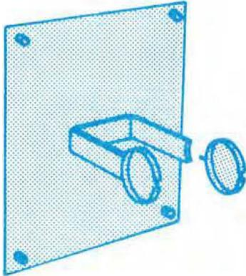
Insert the filter holder with IR-blocking filters in the filter holder on the rear. The filter holder top is marked either X or H. The filter holder X is used for working with the XBO 450W Xenon lamp; for the HBO 200W mercury-vapor pressure lamp, use filter holder H.
