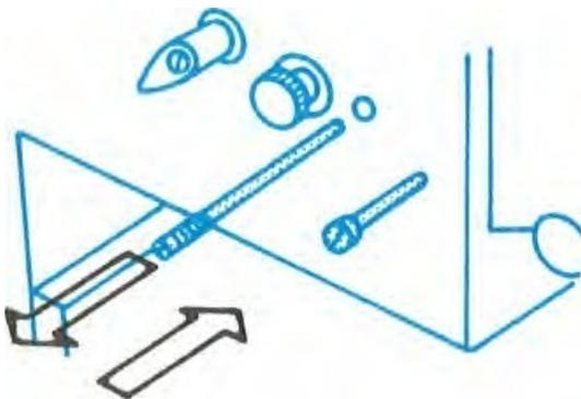
**d)** Remove the red protector on the focus rack, after unscrewing the hex bolt and the slotted screw. Withdraw the protector after the rack is slightly raised. Replace the slotted screw.
