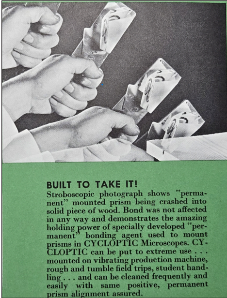
Fig. 5. Photo from 1963 Cycloptic catalog. The bond between the prism and backing plate is claimed to be permanent
