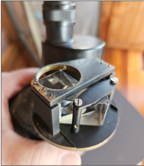
Fig. 4. Inside the head of an older Spencer stereomicroscope with prisms secured with brass brackets
