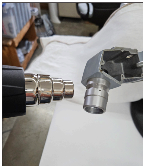
Fig. 14. Using a heat gun to melt the eyepiece tube solder
