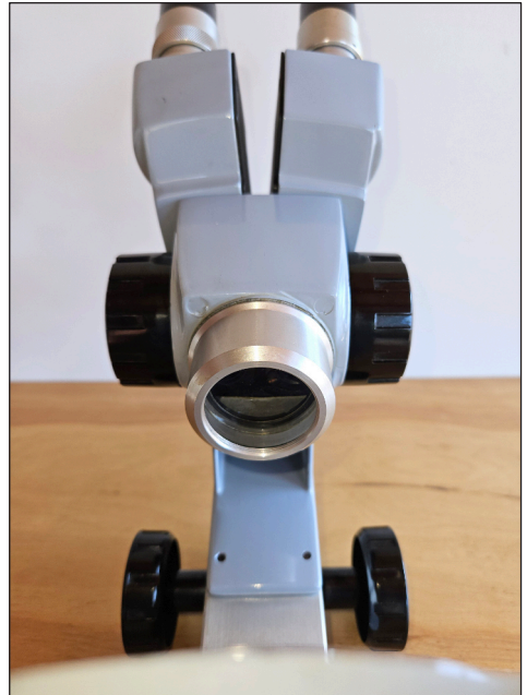
Fig. 3. Cycloptic microscope tilted to show the apochromatic common main objective
