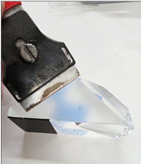
Fig. 11. Removal of trace adhesive from prism
