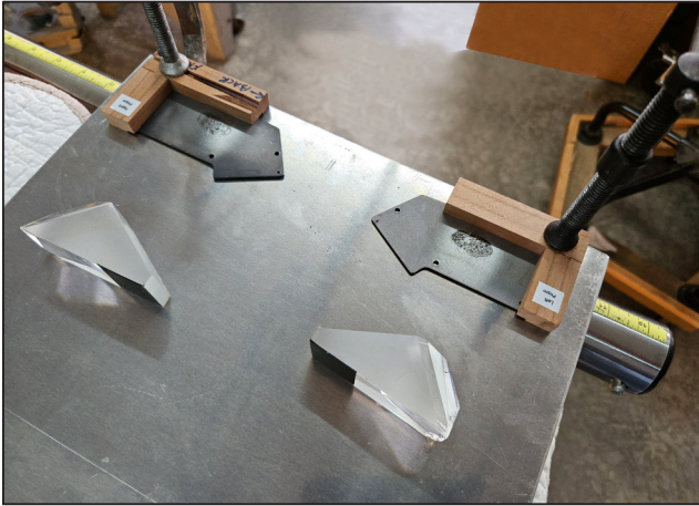
Fig. 15. Jigs prisms and backing plates used for precise alignment during glue up
