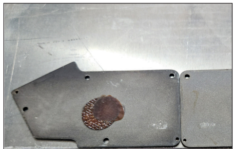
Fig. 9. Backing plates with residual adhesive attached
