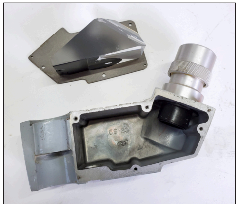
Fig. 8. Prism housing opened to show prism glued to backing plate
