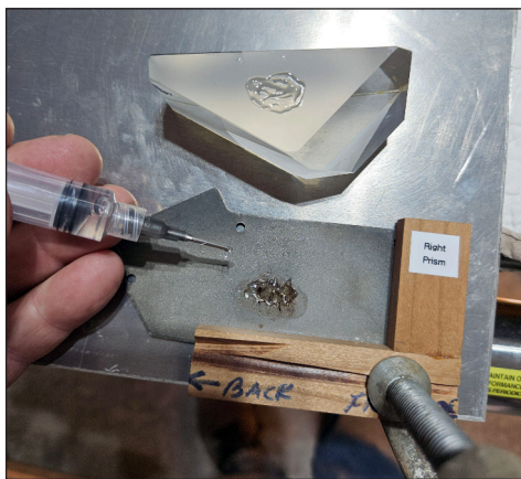
Fig. 18. Applying adhesive to prisms and backing plates
