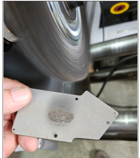
Fig. 12. Removal of trace adhesive with a wire wheel
