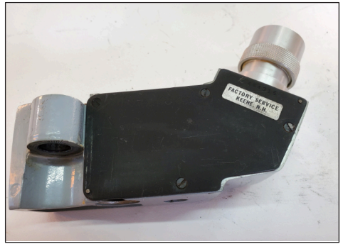
Fig. 7. Prism housing showing unopened backing plate secured with 4 screws
