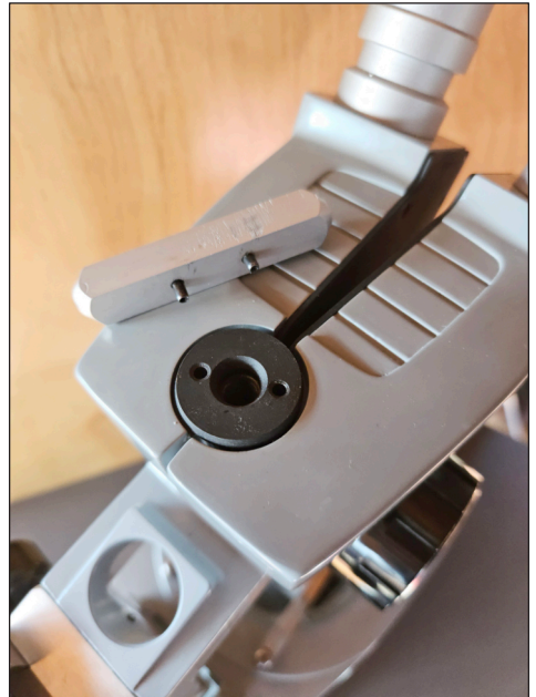
Fig. 6. Cycloptic prism housing bolt and wrench
