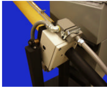
Actuation via DC stepper motor with injector mounted for easy pivoting action
