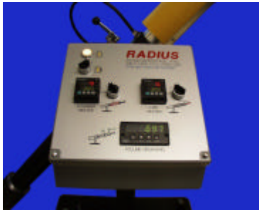
Enclosure control panel for display of temperature and volume remaining
