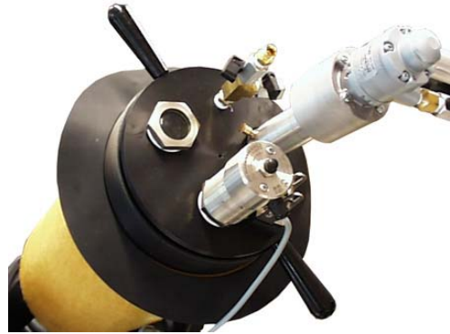
Degassing Unit installed in end of Radius RTM Injector.
