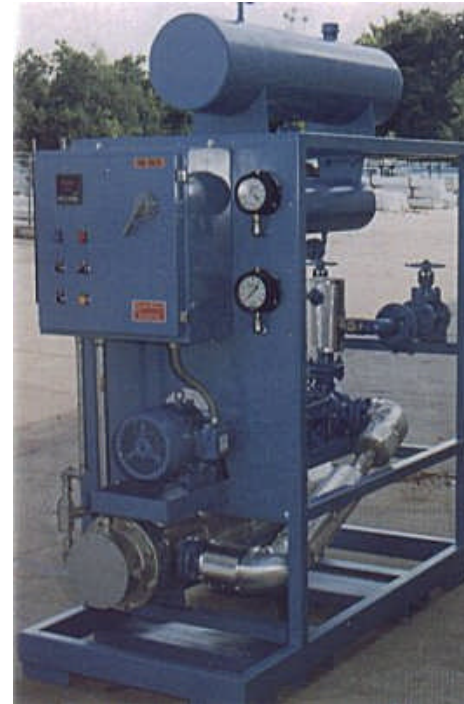
Gaumer 300 kW oil heater w/ 15 hp pump (2.5m x 1.5m x. 2.25m, 1500 kg, 600 l oil reservoir )
