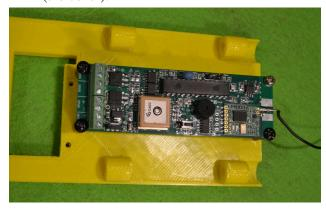
To save weight, many rocket bodies are made from carbon fiber tubing which soaks up all RF. Special dispensation for antennas using external wires or copper tape adhesive are necessary, or, in the case of GPS, a fiberglass window for its signals.
