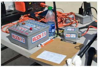
We use multiple launch stations each with its own code and pad number and one controller at the main table. Each pad is powered by a Lithium battery as starting a solid fuel engine and powering the bidirectional communication requires a lot of power. Proper electrical design ensures that the drain of starting (or short) does not interrupt secure communications.
