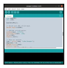
The hardest part of programming any micro-controller is learning the complex input/output systems that vary from manufacturer to manufacturer. The Arduino environment provides software drivers for these systems with a uniform interface. You set the serial port baud rate with Serial.begin(9600); no matter what chip you're using. The details of clocks, port pin setup are taken care of without the tedious, error prone initialization required by an ARM processor or other large MCU.
