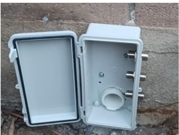
I attached the rubber grommet to the shack-end of the tube, routed the three shack cables through the tube one-by-one from the shack end, then connected them to the bulkhead barrel connectors inside the enclosure. That completed the enclosure construction.
